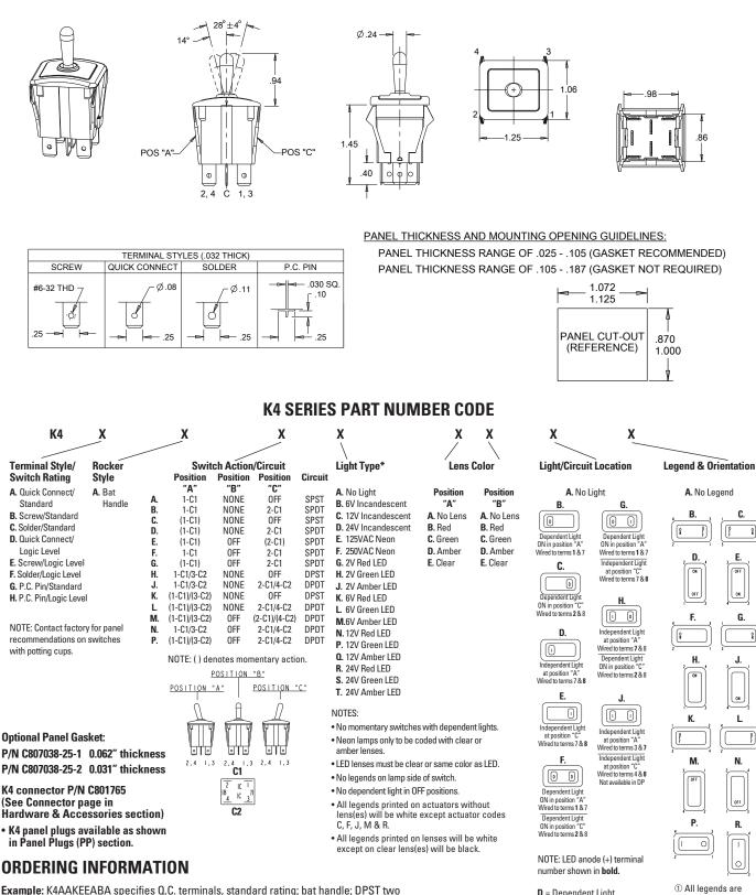
Example: K4AAKEEABA specifies Q.C. terminals, standard rating; bat handle; DPST two position momentary ON, maintained OFF; 125VAC neon light; clear lens in positions "A", no lens in position "C"; dependent light ON in position "A", wired to terminals 1 & 7; no legend.
