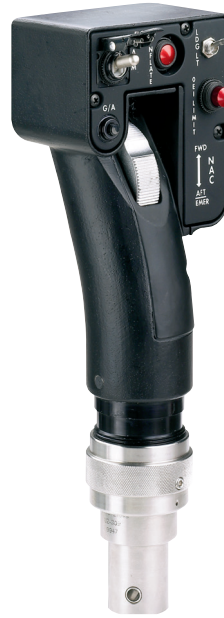
Collective Grip with Thumbwheel Switch and NVG Backlighting
