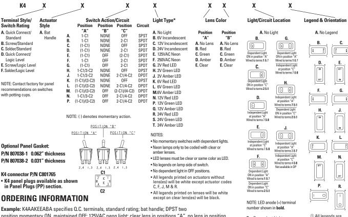
position momentary ON, maintained OFF; 125VAC neon light; clear lens in positions "A", no lens in position "C"; dependent light ON in position "A", wired to terminals 1 & 7; no legend.
