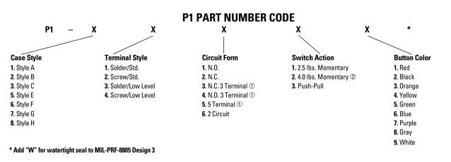
① Circuit styles with 3 and 5 terminals have 50,000 cycle mechanical life per MIL-PRF-8805. ② Military standard is 4.0 lbs.
