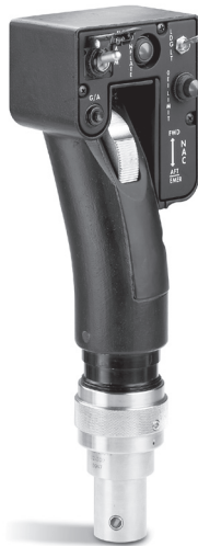
Collective Grip with Thumbwheel Switch and NVG Compatible Backlighting
