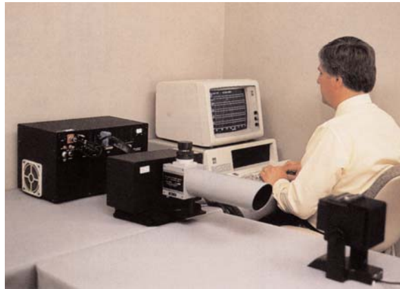
Aerospace Optics spectroradiometer used in measuring and certifying NVIS compatibility.
