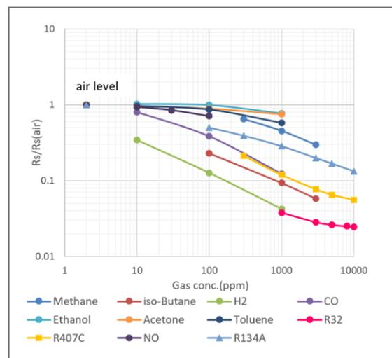
Fig 3. Sensitivity characteristics
