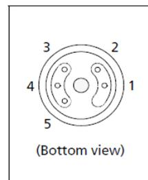
Fig 1c. Pin Layout
