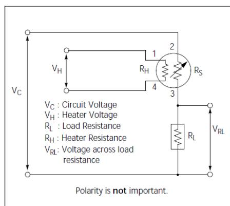
Fig 2. Standard circuit
