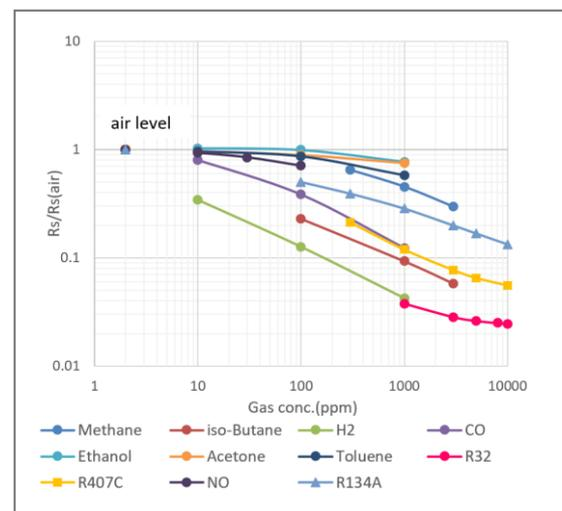
Fig 3. Sensitivity characteristics
